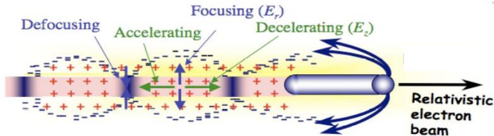
Figure 2. PWFA schematic, indicating plasma oscillations set up by drive electron bunch expelling plasma electrons from the path of the drive bunch.
