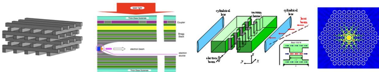
Figure 4. Left to right: examples of the woodpile, MAP, grating, and photonic band gap fiber accelerator structures.
