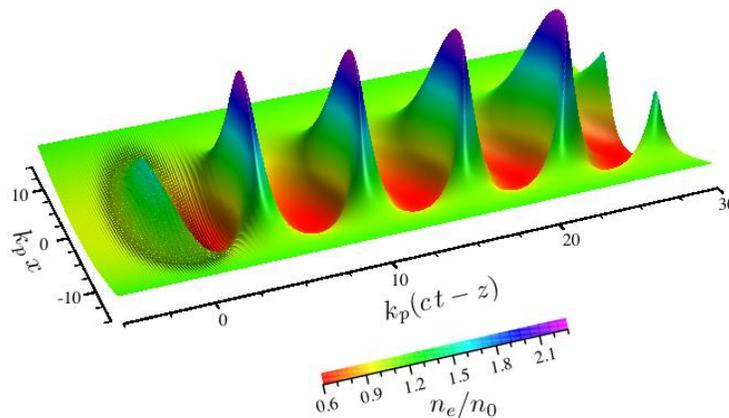
Figure 1. Numerical simulation of a large amplitude plasma wave (plasma electron density perturbation) generated by an intense laser pulse, with electrons trapped in the wave being accelerated.
