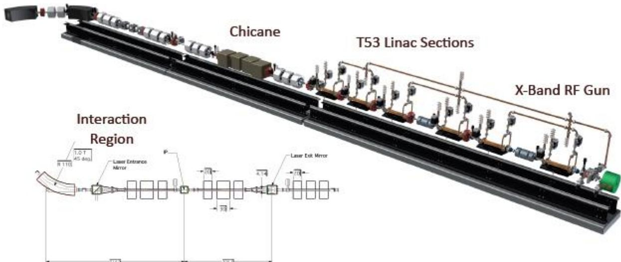
Figure 7. Schematic of the LLNL 2.2-MeV light source.
