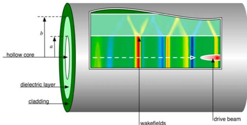
Figure 3. Wakefields set up by the interaction of a drive beam with a dielectric liner. The Cherenkov cone is seen in the dielectric.
