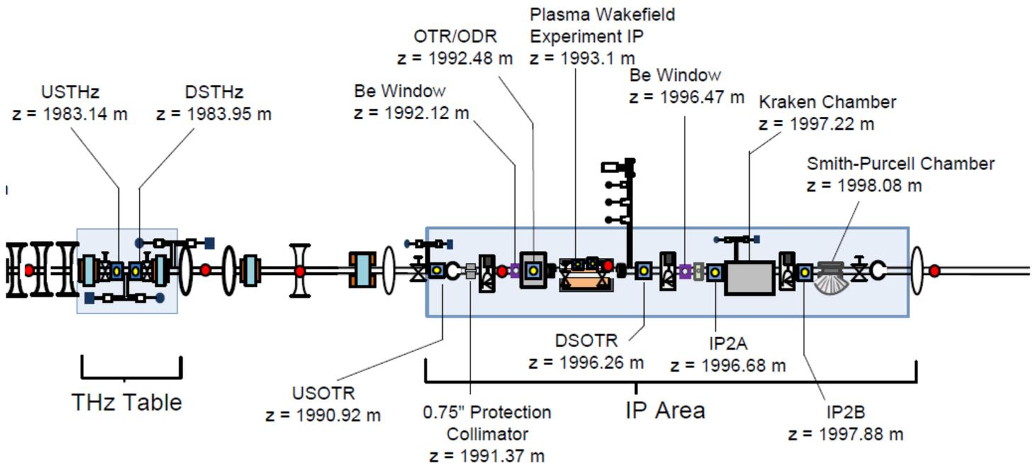
The “Kraken” is a massive multi-port vacuum chamber for use by experimenters on the second “IP” table. At this location the beam can be focused to a small spot.
