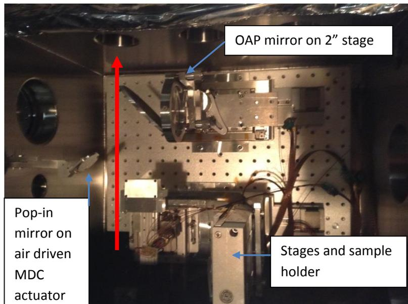
Figure 2: Photograph of contents of Kraken for E-201. The red arrow shows the beam path.
