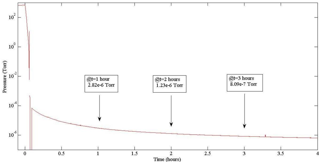
Figure 3: Pump down plot from atmosphere of Kraken with Agilent TPS with New Generation Turbomolecular Pump Turbo-V 81-M.
