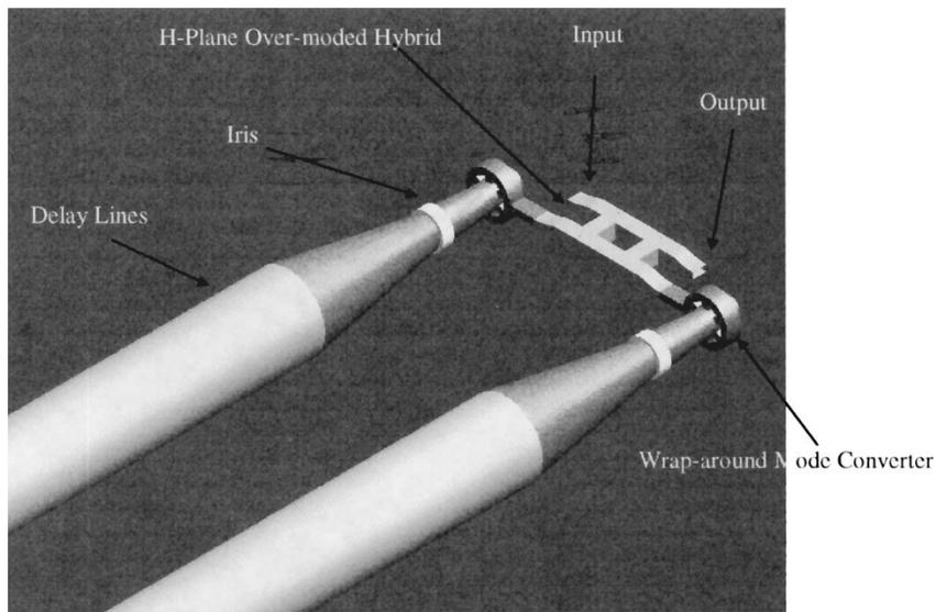
Fig. 4. Resonant delay-line pulse-compression system.
