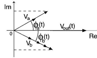
Fig. 2. Phasor diagram showing the voltage during the compressed pulse as composed of contributions from six time bins, phase modulated so as to form two phasors rotating in time. Cancellation of the imaginary parts is maintained while the sum of the real parts yields a constant-phase output voltage of changing amplitude.
