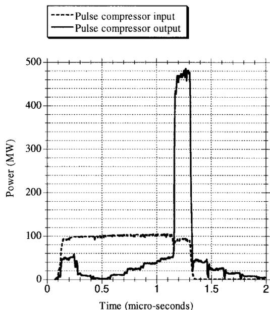
Fig. 14. High-power input and output signals. The output pulse has a power level in excess to 470 MW.
