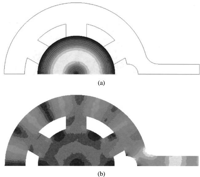
Fig. 6. HFSS simulation results for the wraparound mode converter. The different shades represent the magnitude of the electrical field. (a) A cut plane through the slots. (b) A cut plane in the circular guide 2.5 cm away from the slots.
