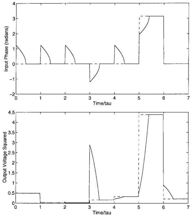
Fig. 3. Pulse shaping with resonant-delay-line pulse compression. The beginning portion of each time bin is phase modulated with one of two functions (in addition to the phase flip). The compressed output pulse acquires a ramp. The missing energy in this example is largely moved to the fourth time bin of the output waveform. Dashed lines show the corresponding waveforms without pulse shaping.
