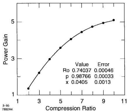
Fig. 13. The points are measured power gains for different compression ratios. The curve represents the least squares fit for the parameters in (28) with values as shown in the table.
