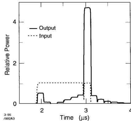
Fig. 12. Pulse compressor output for a compression ratio of eight: input pulsewidth of  $1.2 \mu\text{s}$  and output pulsewidth of  $0.15 \mu\text{s}$ .
