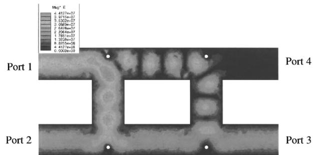
Fig. 9. HFSS simulation results of the  $H$ -plane hybrid. The different shades represents the magnitude of the electrical field. Port 1 is being excited. Note that Port 1 is completely isolated from Port 2.
