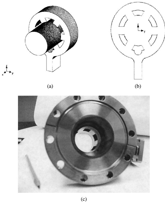
Fig. 5. Wraparound mode converter. The physical model shown does not have the back-wall shorting plate, this is done for illustration purposes only.
