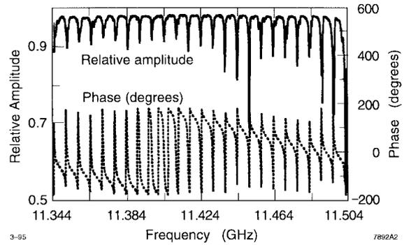
Fig. 11. Pulse compressor measured frequency response in magnitude and phase.
