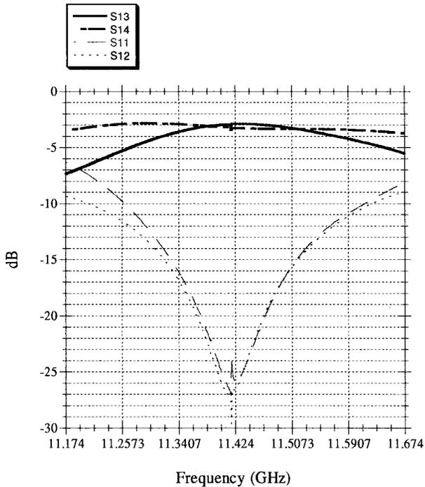
Fig. 10. Cold test measurements of the  $H$ -plane hybrid. The parameters of the hybrid were optimized at 11.424 GHz.
