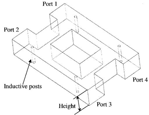
Fig. 8. Schematic diagram of the over-moded  $H$ -plane hybrid.
