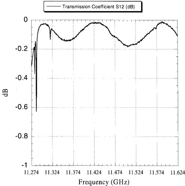
Fig. 7. Transmission coefficient for two wraparound mode converters back to back. The device is optimized at 11.424 GHz.
